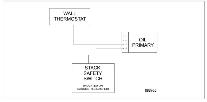
Figure 4P - Stack Safety Switch Wiring Diagram
