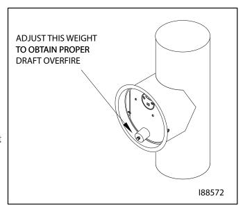
Figure 8B - Adjustment of Barometric Damper
