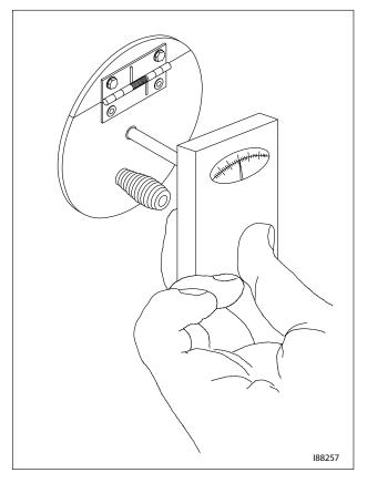
Figure 8A - Checking for Proper Draft Over Fire
