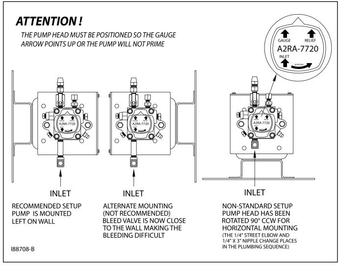
Figure 4I - Proper Positioning of Metering Pump Head
