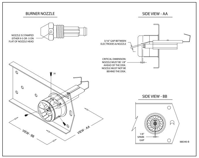
Figure 3E - Burner Nozzle and Electrode Specifications
