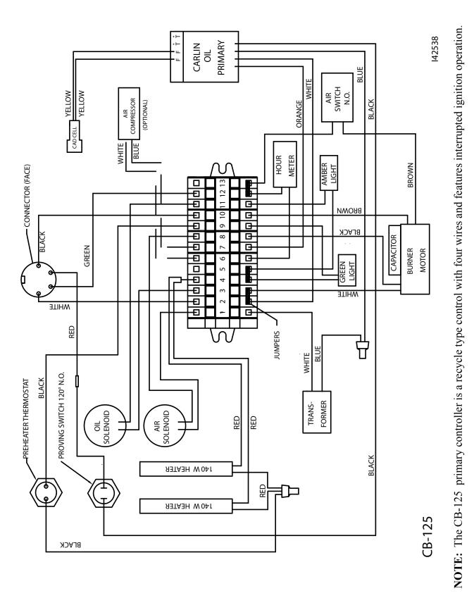
FIGURE B2 - CB-125 Burner Wiring Diagram
