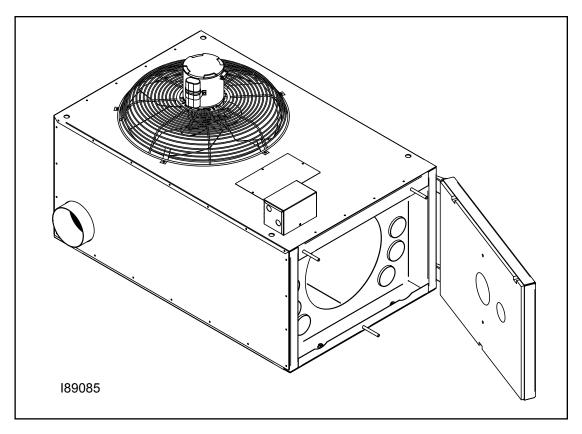
Figure 2A - Accessing the Combustion Chamber
