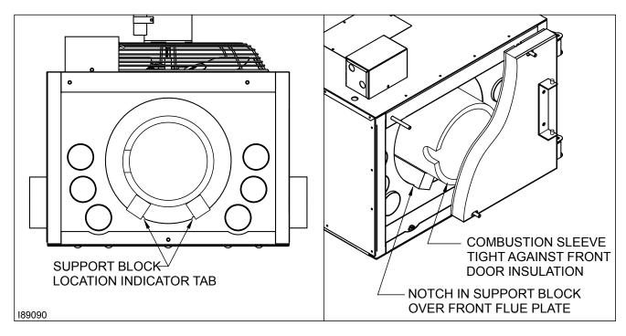
**Figure 3D - Installing the Combustion Sleeve**
