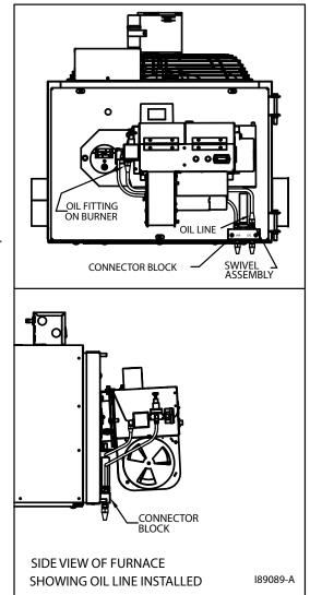
Figure 3F - Installation of Connector Block and Oil Line
