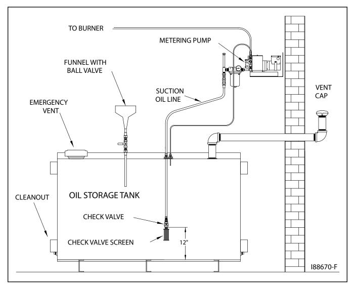
Figure 9C - Check Valve Detail
