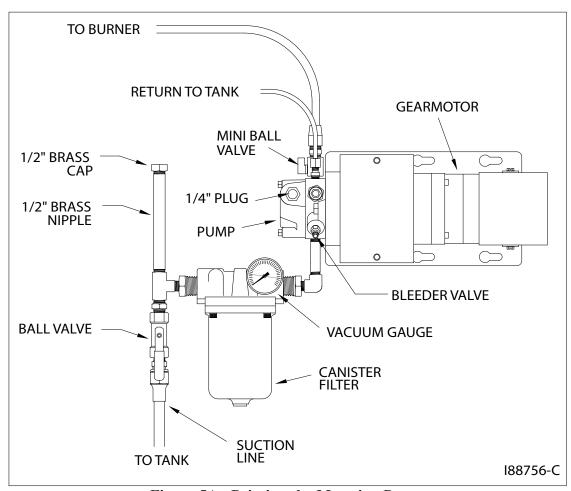
Figure 5A - Priming the Metering Pump
