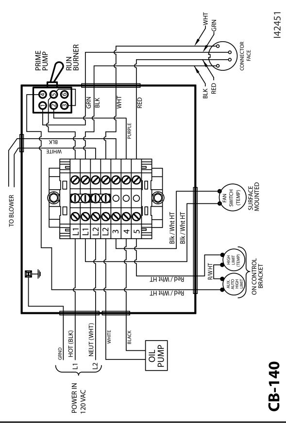
FIGURE B1 - CB-140 Furnace Wiring Diagram
