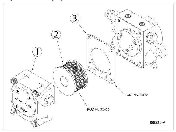
Figure 9B - Servicing the Metering Pump
