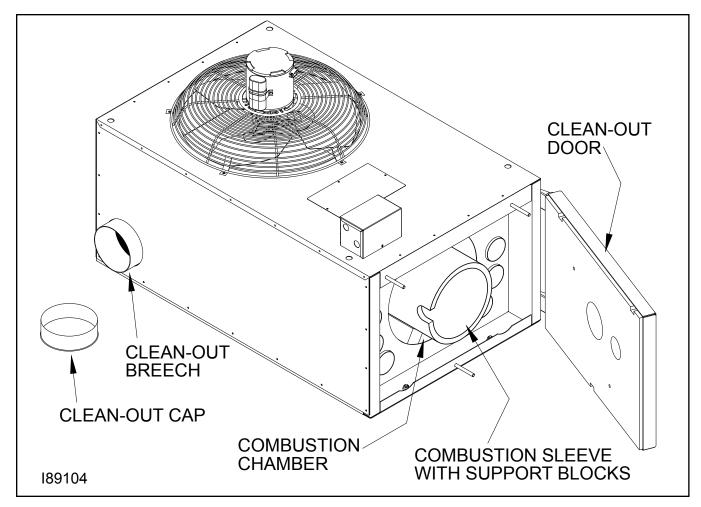
Figure 9D - Accessing the Combustion Chamber for Cleaning
