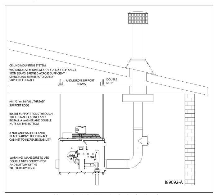
Figure 4C - Ceiling Mounting Installation Overview
