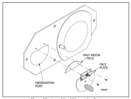
Figure 3B - Assembly of Observation Port
