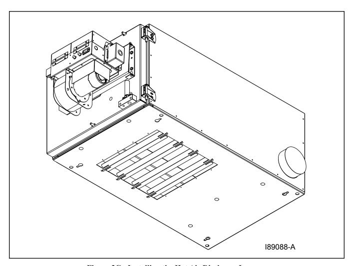
Figure 3C - Installing the Hot Air Discharge Louvers
