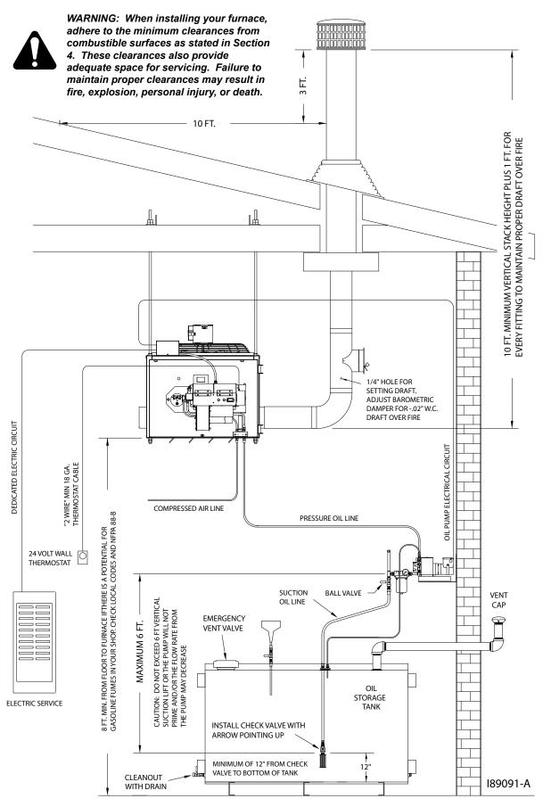
Figure 4A - Typical CB-140 Furnace Installation
