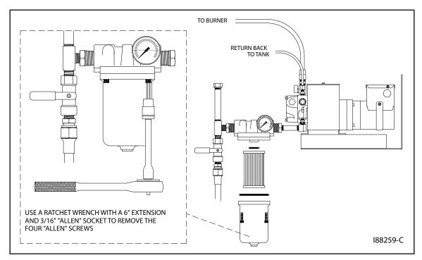
Figure 9A - Canister Filter Component Detail
