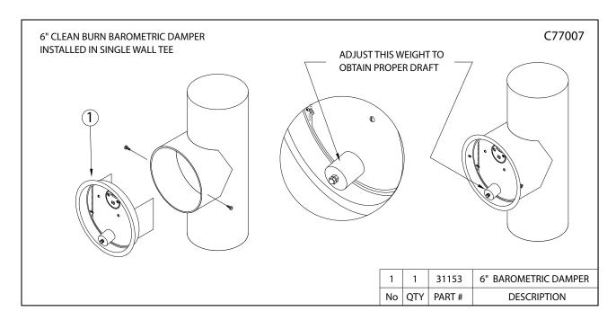
Figure 4N - Installation of Barometric Damper
