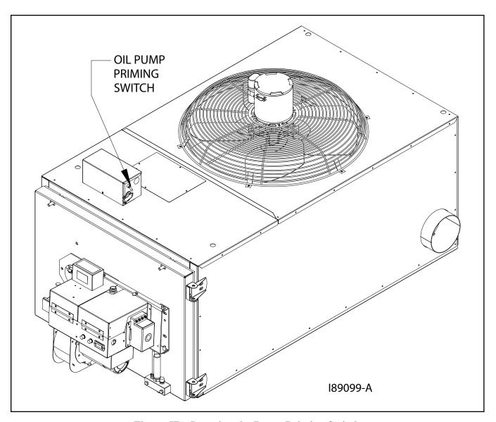
Figure 5B - Locating the Pump Priming Switch
