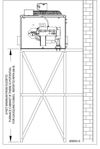
Figure 4D - Furnace Installed on Raised Platform
