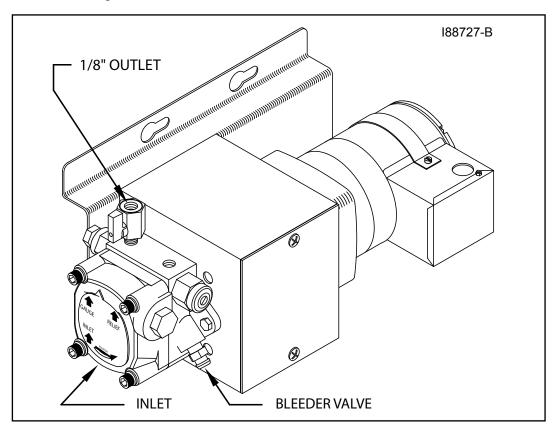
Figure 4G - Vertical Mounting of the Metering Pump
