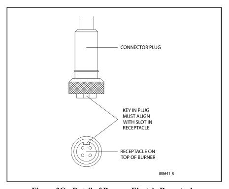
Figure 3G - Detail of Burner Electric Receptacle
