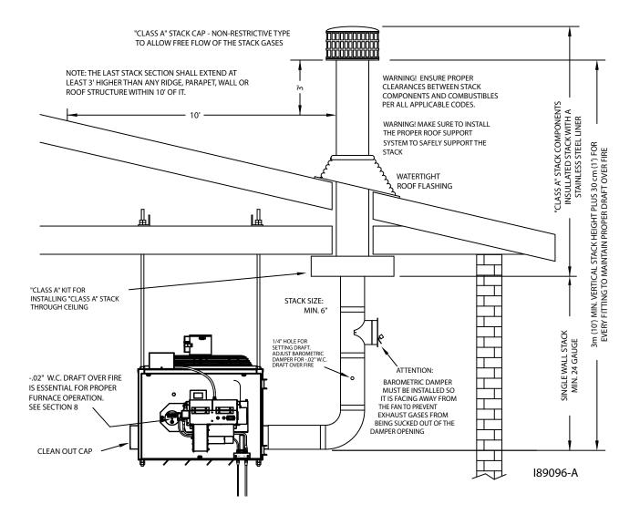
Figure 4L - Installation of "Class A" Stack Through Roof/Ceiling
