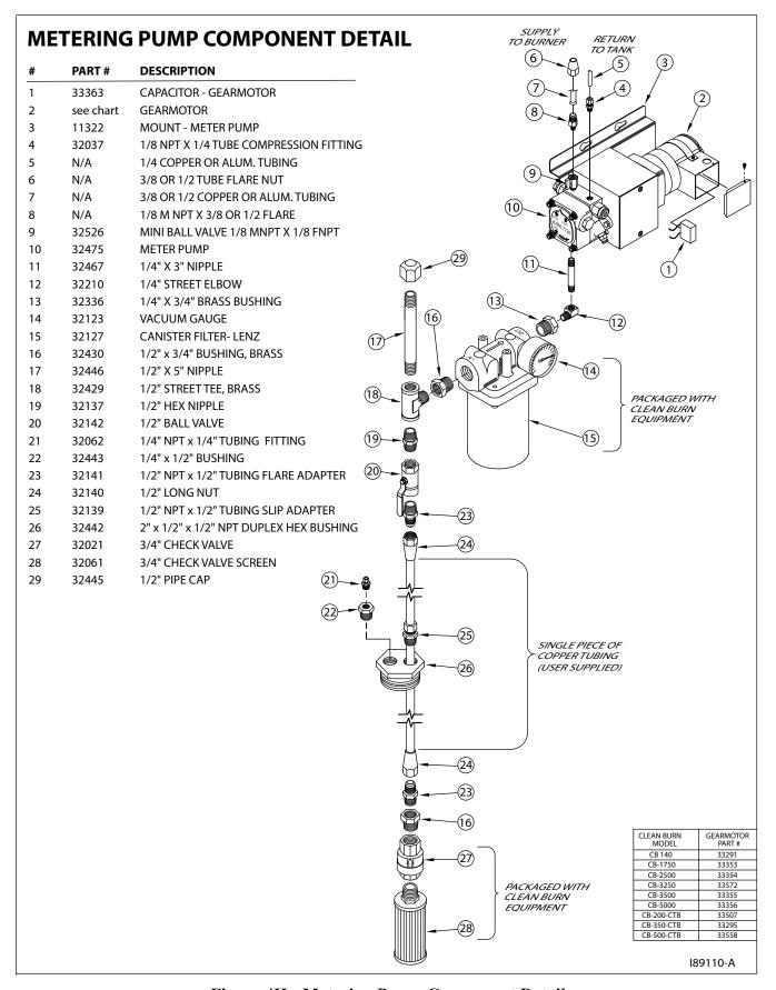
Figure 4H - Metering Pump Component Detail
