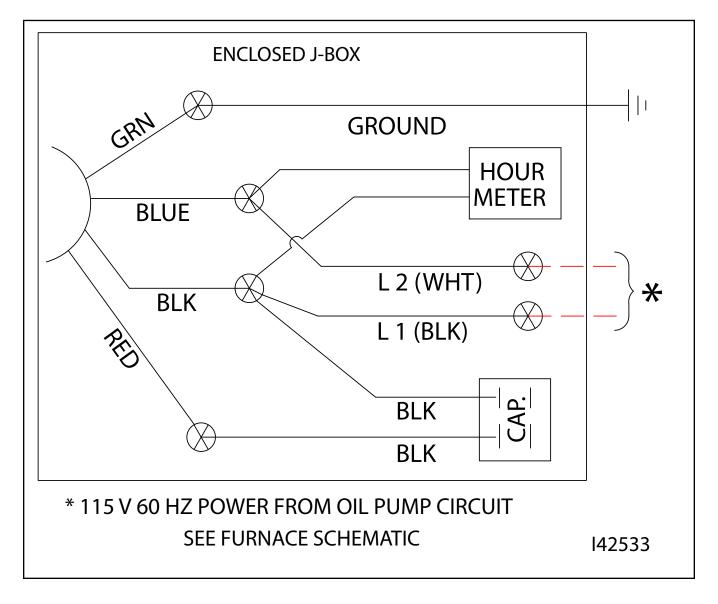
**Figure B4 - Metering Pump Wiring Schematic**
