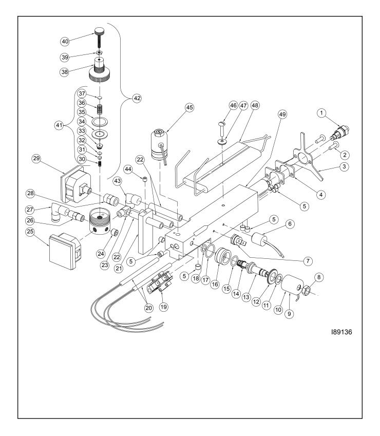
FIGURE A2 - Preheater Block Assembly Component Detail
