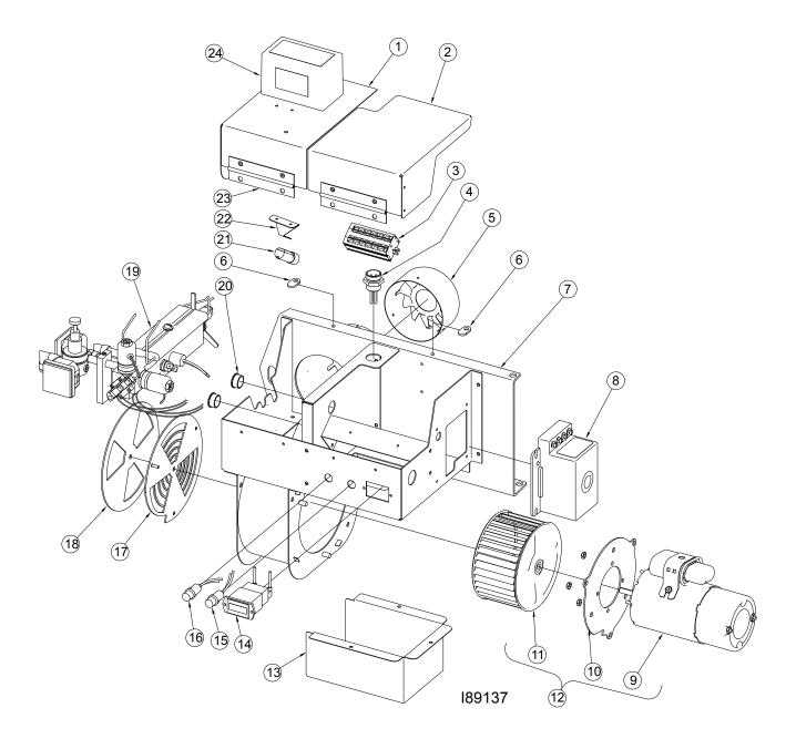
FIGURE A1 - Burner Component Detail
