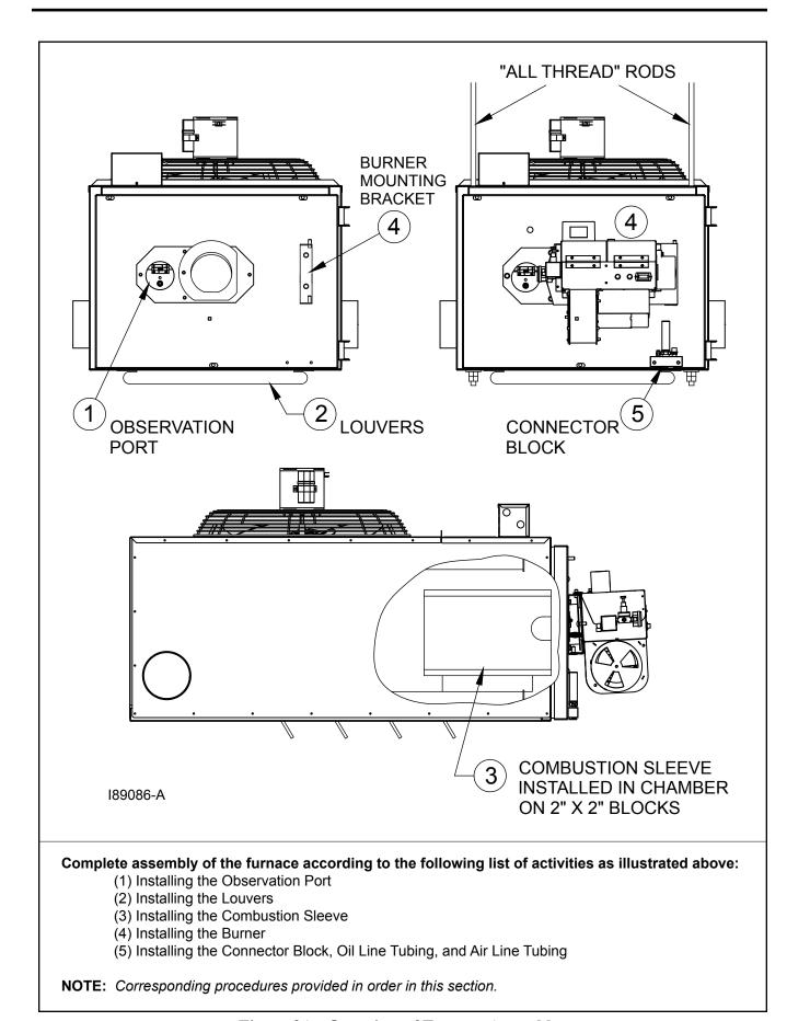
Figure 3A - Overview of Furnace Assembly
