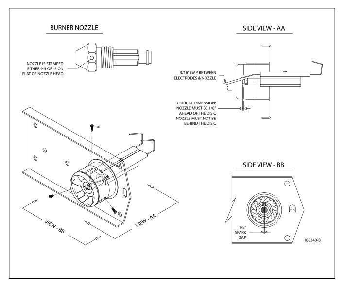
FIGURE A3 - Burner Electrode Component Detail
